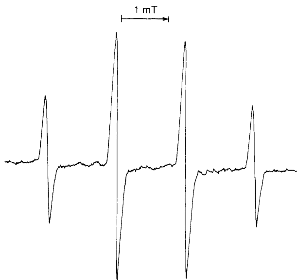
Fig. 1 ESR spectrum of DMPO-OH adduct generated from \text{Cu}^{\text{II}}(\text{en})_2 - \text{H}_2\text{O}_2 system in the presence of DMPO at pH 7.4. Reaction conditions: \text{Cu}^{\text{II}}(\text{en})_2 , 0.001 \text{ mol dm}^{-3} ; \text{H}_2\text{O}_2 , 0.1 \text{ mol dm}^{-3} ; DMPO, 0.05 \text{ mol dm}^{-3} .
